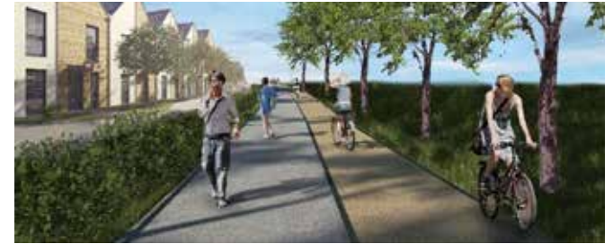
Commuter cycle routes approx 2.5m wide with segregated footpath total approx width 4.6m
