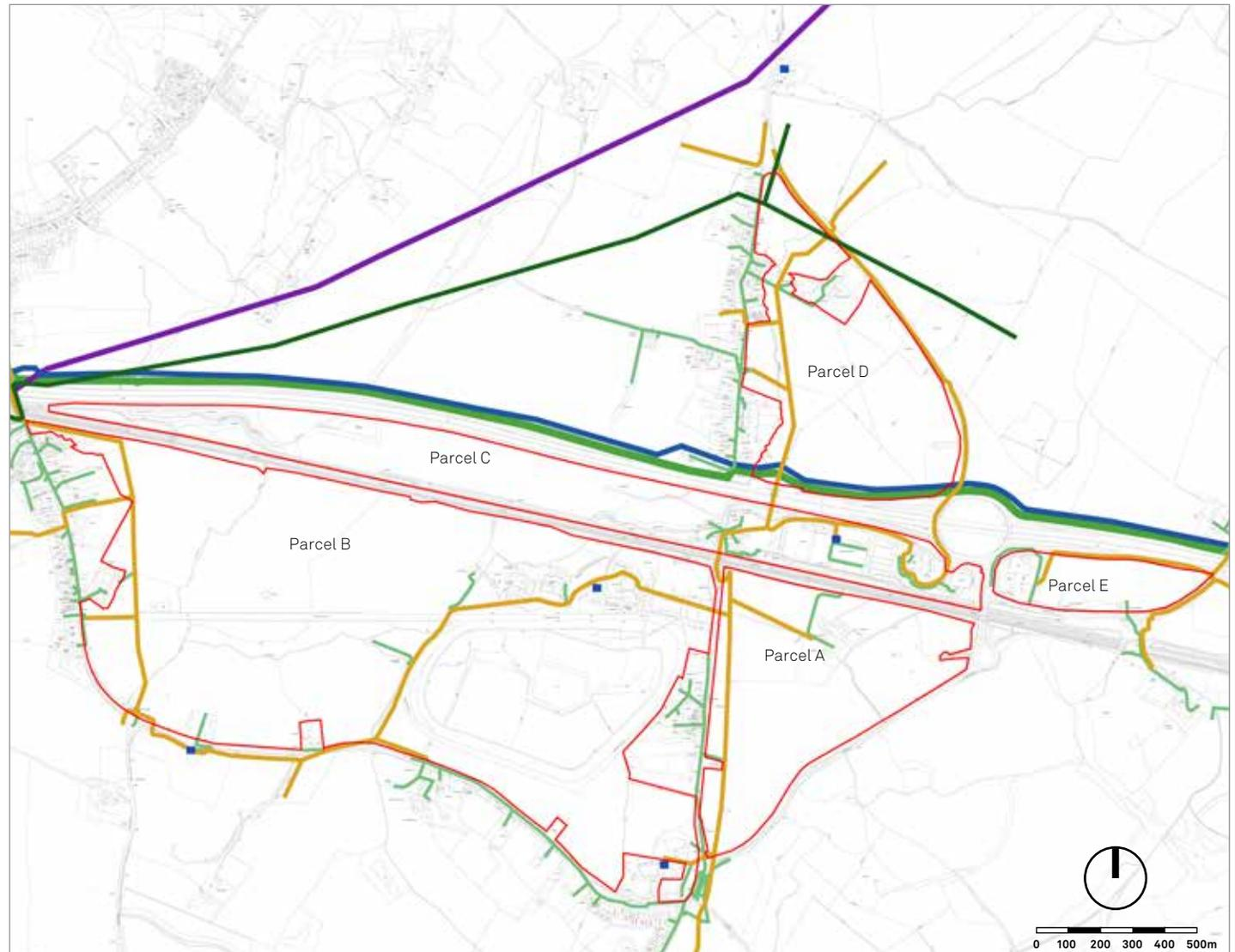
**Figure 2.13: Existing electricity apparatus within and adjacent to the study area**
