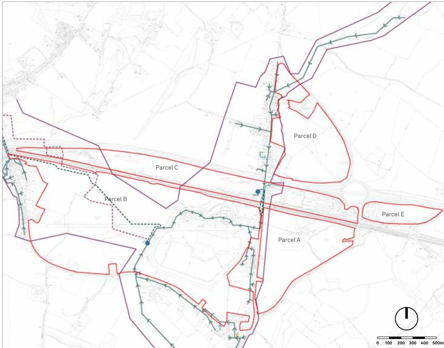
Figure 2.16: Existing foul water apparatus within and adjacent to the study area
