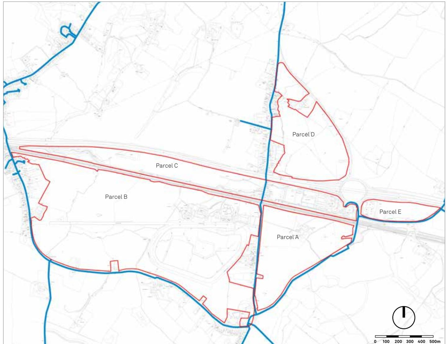
Figure 2.15: Existing potable water apparatus within and adjacent to the study area
