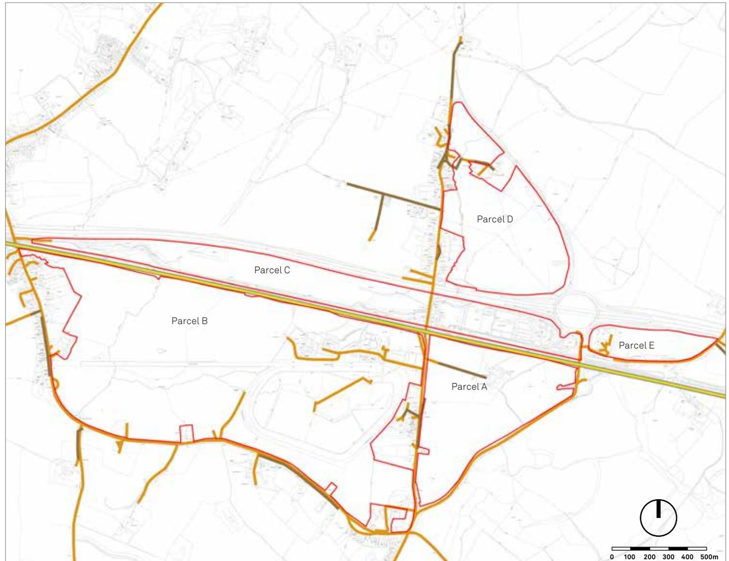
Figure 2.17: Existing telecommunications apparatus within and adjacent to the study area
